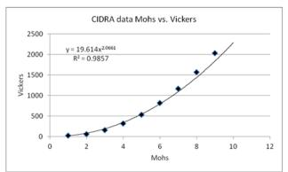
Figure 1: CIDRA data for Mohs vs. Vickers
